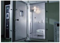
Temperature & Humidity Cycle Test Chamber
