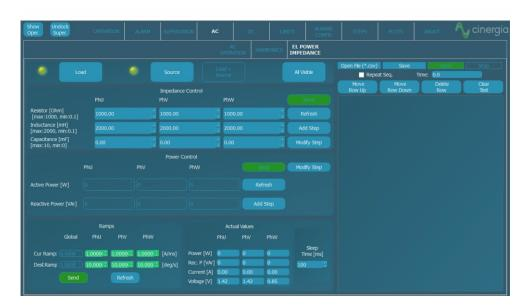
Power and Impedance Control In Power mode, the active and reactive power of each phase is independently controlled. In Impedance mode, the device emulates an RLC load allowing to parameterize resistance, inductance and capacitance per phase making this device suitable for Anti-Islanding test of grid converters.
