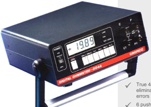
The DO4A is a practical instrument for low resistance measurement, ideal for use in the workshop, field or test facilities. It is of rugged construction contained in an aluminium case with tilt handle. The DO4A has many advanced features, including protection up to 415 volts rms. digital calibration and long scale length, (4000 count.)
