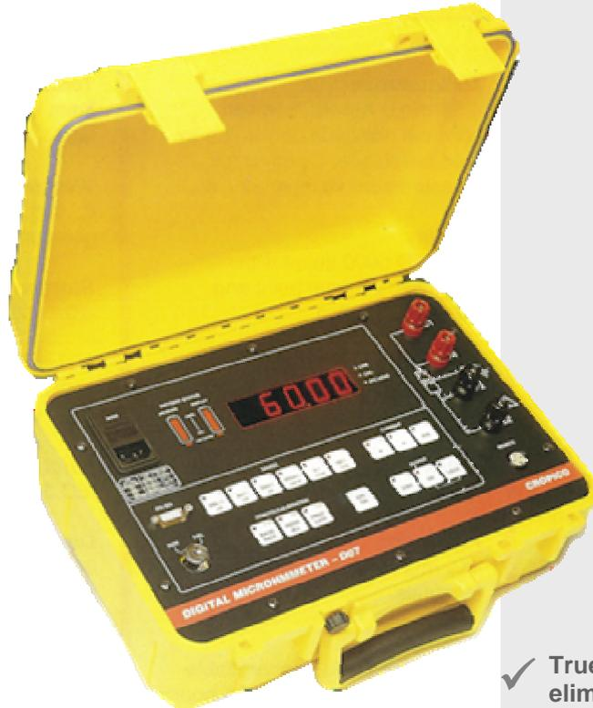
The DO7 is a very rugged yet compact and portable digital microhmmeter for the measurement of low resistance. Using a rechargeable sealed lead acid battery with built-in charger the DO7 is capable of measuring with a current of 10Amps on the lowest range.
