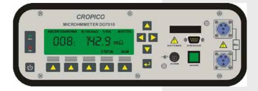
The DO7010 is a very rugged and very compact, portable digital ohmmeter for the measurement of low resistance. Using rechargeable and replaceable NiMh batteries with external charger the D7010 is capable of measuring with a current of 1 and 10Amps on all except the highest range.
